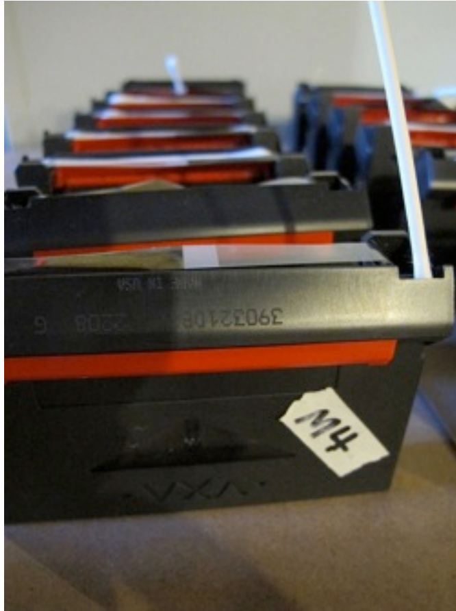
A VXA data tape with a recovery identifier, intended to match it up with its case (labeled with the same id) after drying.
