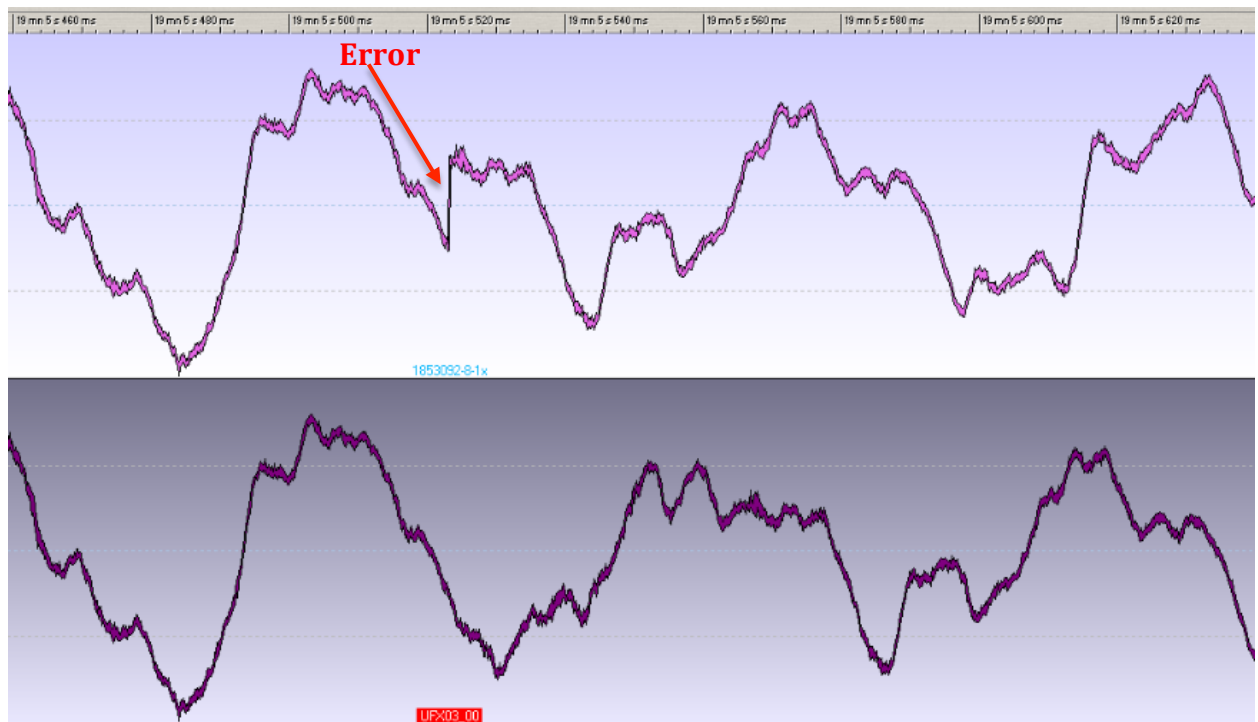
Figure 1: DAW file with interstitial error (Top Waveform) compared to the intact Reference file (Bottom Waveform)
